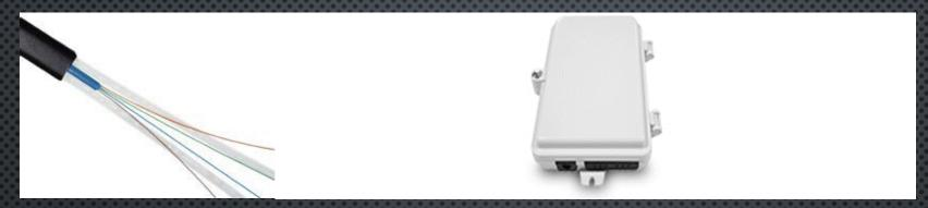
This cable in a 2F version costs about 20 cents a meter. It comes on 4 Km spools and is used to connect a premises box like you see here to a splice case that links 12 of these to a 24F cable. The big magic is that unlike wire cables, optical fibre carries what you decide to put into it.
